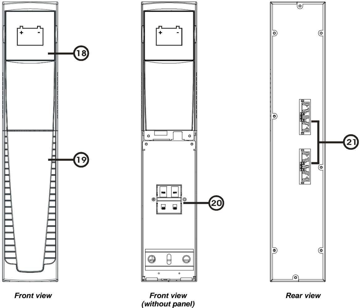
**18** Extractable/ rotatable battery box plate
