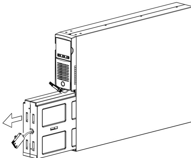
5. Insert the new battery pack into the compartment, sliding it into the UPS. Put the battery pack retention panel back in position and secure it with the two screws removed previously. Connect the battery pack cable to the UPS and close the front panel. Set the UPS to normal operation mode by pressing ON + SEL for at least 4 seconds.
