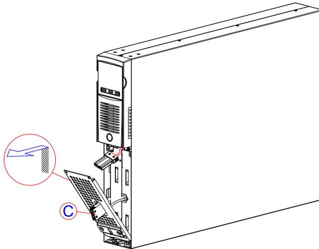
4. Slip off the battery pack pulling it towards the outside, as shown in the figure below. Be careful when extracting and lifting up the battery pack as it is heavy.. ATTENTION: the new battery pack must contain the same number and type of batteries (see the label located on the battery pack near the connector).
